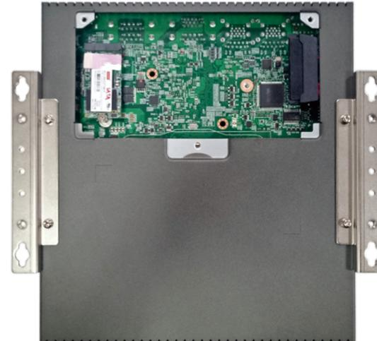
3. Place the thermal pad (included in the accessory bag) on top of the module.
