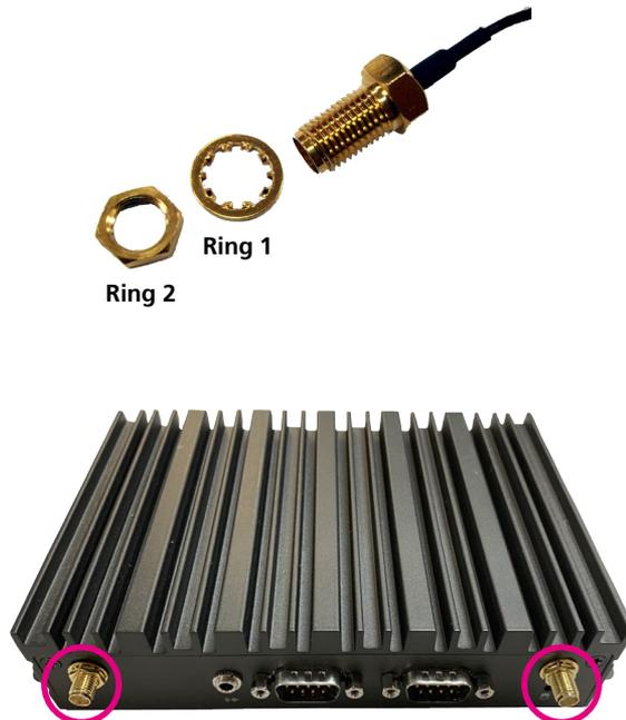
4. Connect the external antennas to the Wi-Fi antenna jacks.
