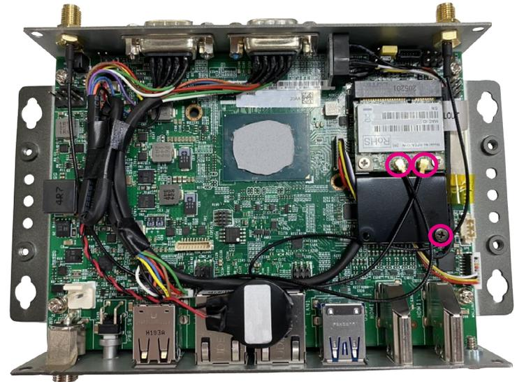
3. Insert the 2 rings (ring 1 then ring 2) into the Wi-Fi antenna jacks. Please remove the two antenna hole covers on the front panel before installing the antenna jacks.
