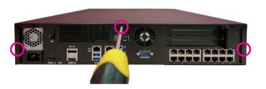
2. Push the chassis top cover forward until it fits snugly with the chassis.
