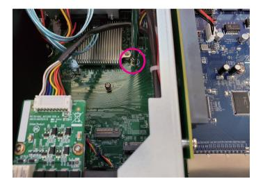
2. Insert the M.2 module into the M.2 Key M slot at a 45-degree angle until the gold-plated connector on the edge of the module completely disappears into the slot.
