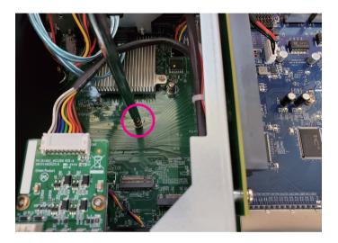
2. Insert the M.2 module into the M.2 Key B slot at a 45-degree angle until the gold-plated connector on the edge of the module completely disappears into the slot.
