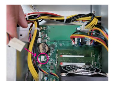
10. After connecting the power, use cable ties to organize the cables.
