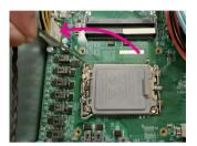
3. Lift the CPU load plate up to open the socket completely.
