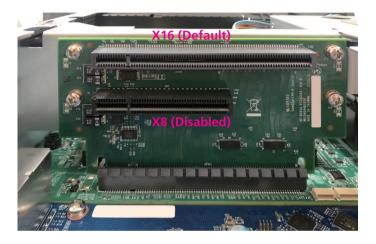
4. The usage mode for these two slots depends on the settings configured in the BIOS. If the BIOS is in 1x16 mode, the upper slot will operate in x16 mode, while the lower slot will not be available. Conversely, both slots will operate in x8 mode when selecting 2x8 in the BIOS, and the bandwidth of the upper slot (x16) will be split and shared with the lower slot. By default, the BIOS is set to x16 mode.
