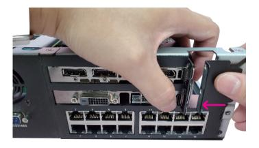
5. Using the screws you set aside in step 1 to firmly secure both the brackets and the graphics card in place.
