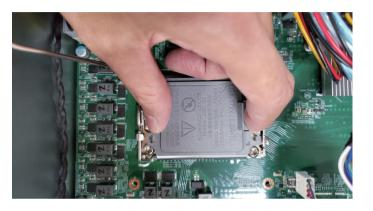
6. Gently push the load lever down until it locks under the retention tab.
