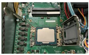
5. Slightly close the load plate and remove the plastic cover from the load plate.
