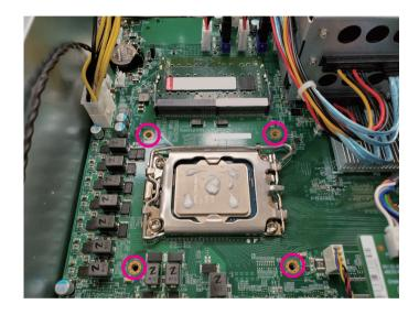
8. Place the heatsink module in position, aligning it with the mounting holes mentioned in the previous step on the mainboard. Tighten the screws following the order marked in the image below.
