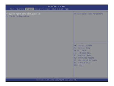
2. Within the Chipset tab, locate the System Agent (SA) Configuration, and then find the setting for PCle slots (X16 Mode Select).
