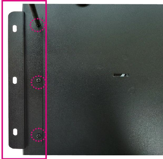
4. Use the screws to lock the other bracket side onto the device.
