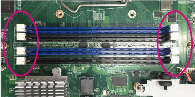
2. Insert the module into the socket at a 90 degree angle. Apply firm even pressure to each end of the module until it slips into the socket.
