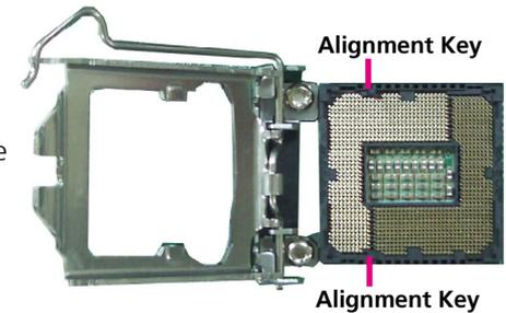
The CPU's notch will at the same time fit into the socket's alignment key.
