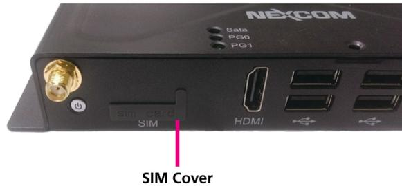
2. Insert the SIM card into the slot.
