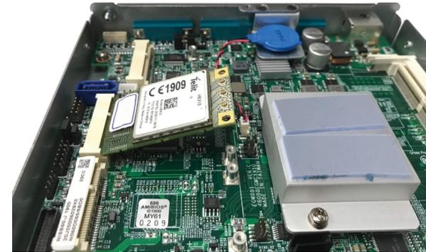
3. Push the module down and then secure it with mounting screws.
