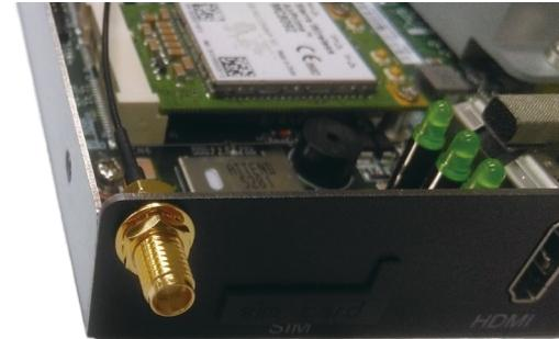
3. Attach the RF cable onto the module.
