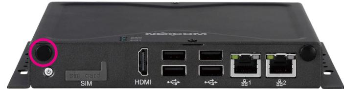
2. Insert the SMA antenna jack end of the cable through the antenna hole, and insert the 2 rings (ring 1 and ring 2) back to the antenna jack.
