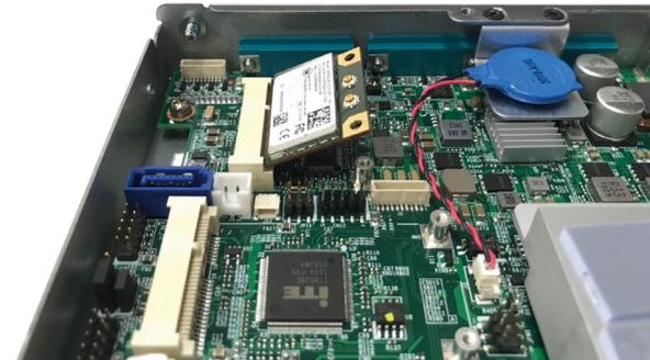
3. Push the module down and then secure it with mounting screws.
