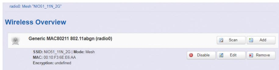
To set up the Wireless configuration, please select “Network” in the tab, then select “WiFi”, which would show you the current status of radio interfaces.
