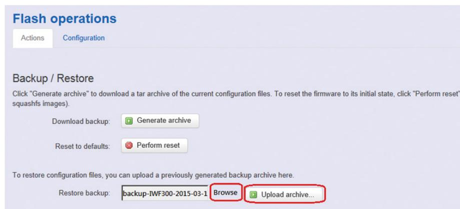
**Note:** After restoring the file, the system will apply the changes and reboot automatically. Due to the settings from configuration backup, the IP address may change and you have to enter the new IP address accordingly. Otherwise, the new web page may not be accessible.
