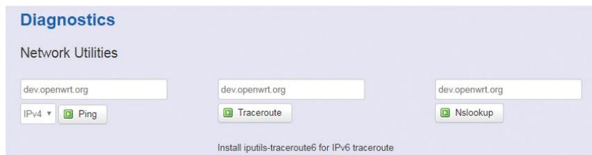
**Ping:** Test the reachability of a host on an Internet Protocol (IP) network and measure the round-trip time for messages sent from the originating host to a destination host and back. The only required parameter is the name or IP address of the destination host.
