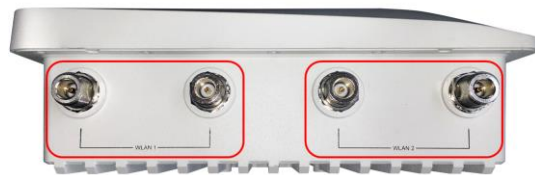
Wi-Fi antenna connector for Wi-Fi Mesh connection (WLAN 1 & WLAN 2)
