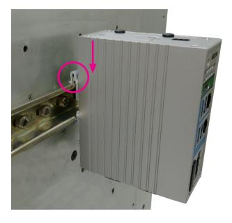
4. Push NIFE 105 back to connect the bracket with the DIN rail and complete installation.
