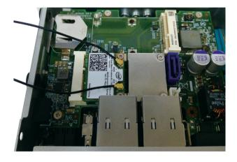
2. Locate the antenna holes on the top panel and insert the antenna jacks through the antenna holes. Fix the antenna jacks with ring 1 then ring 2.
