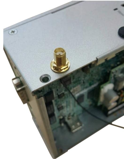
3. Connect an external antenna to the antenna jack.
