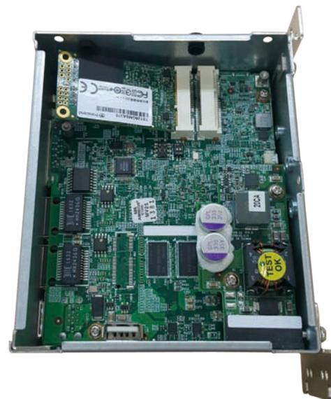
3. When installing a 3G module, make sure to install the SIM card first.
