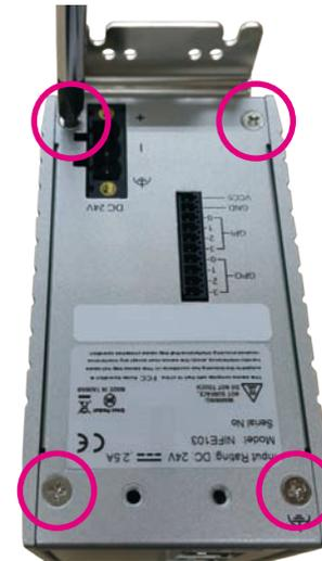
3. Remove the screws on the rear chassis.
