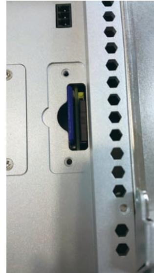
5. Press down the SD card until it is fixed into the socket.
