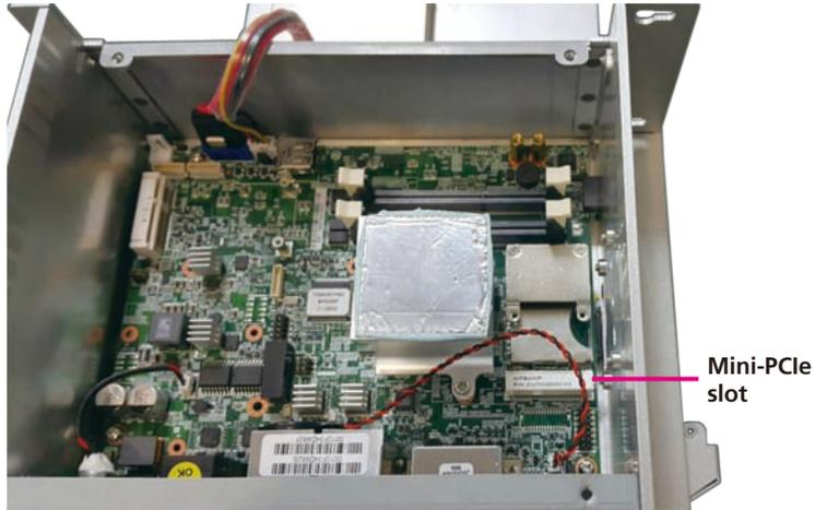
2. Remove the mini-PCle bracket from the board.
