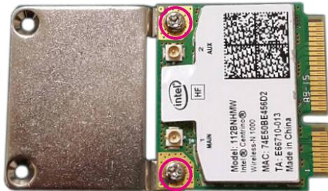
4. Insert the mini-PCIe module into the mini-PCIe slot at a 45 degree angle until the gold-plated connector on the edge of the module completely disappears into the slot.
