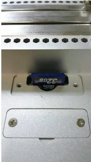
4. Ensure the SD card is correctly secured in position.
