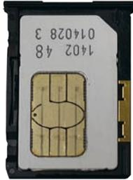
8. Insert the SIM card holder back to its original position.
