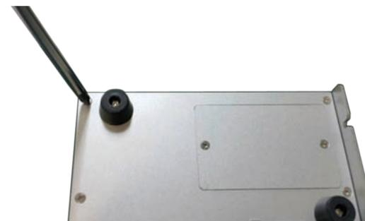
3. Locate the two screws on the side cover. (Four screws for NET 200-ECM)
