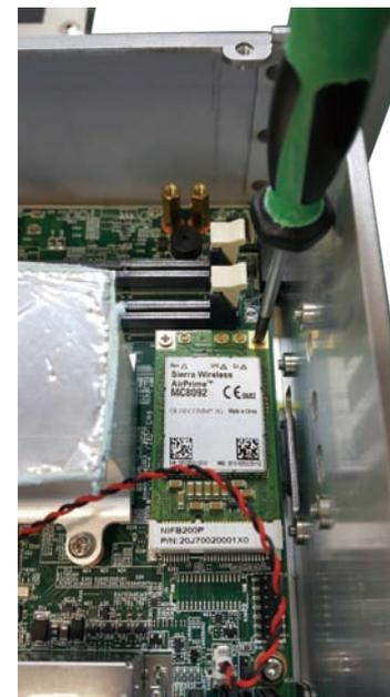
2-2. Secure the module with screws.
