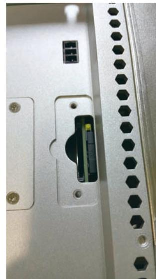
3. Insert the SD card into the SD card socket.
