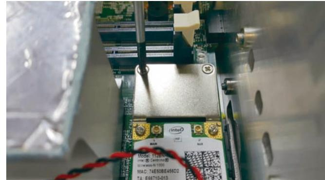
5. Push the module down and secure it with screws.
