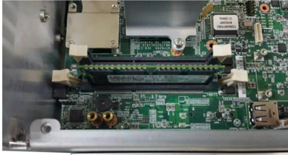
6. Ensure the memory module is secured properly into the socket.
