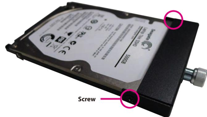
4. Put the HDD back into the slot gently, then tighten the screw to secure it.
