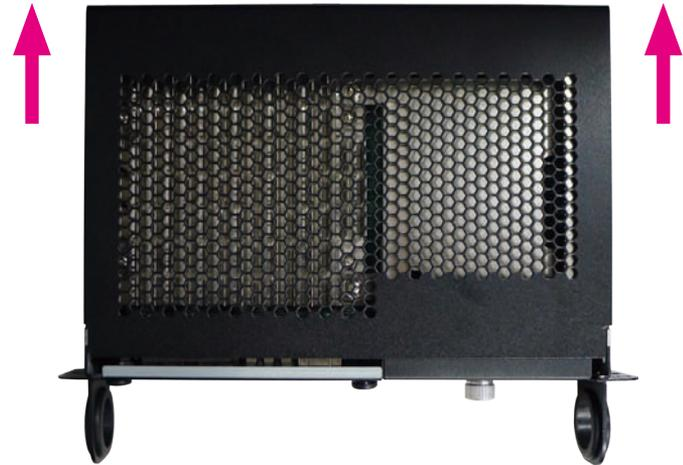
2. Remove the screws securing the HDD bracket and then remove the bracket.
