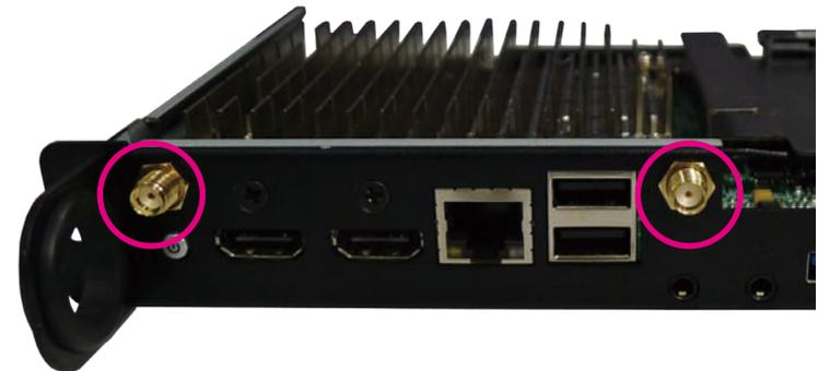
7. Connect the external antennas to the Wi-Fi antenna jacks.
