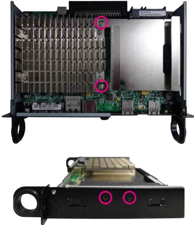
3. Locate the NGFF slot and insert the NGFF SSD module into the slot.
