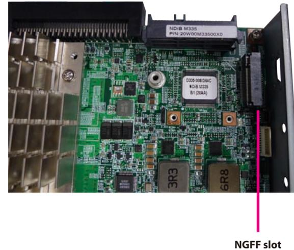
4. Fasten a screw into the standoff to secure the NGFF SSD module.
