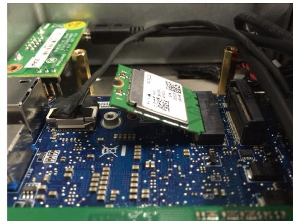
3. Secure the module with mounting screws.
