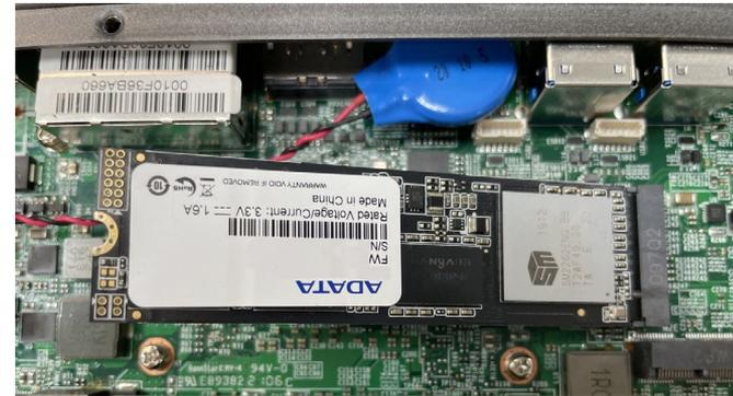
3. Push the module down and secure it with the screw that was removed from step 1.
