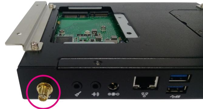
5. Connect the external antennas to the Wi-Fi antenna jacks.
