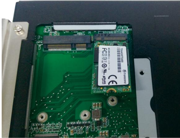
3. With the module fully inserted, tighten a screw into the mounting hole on the module to secure it.
