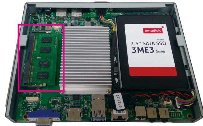
3. Open the bottom cover for installing the 2nd SO-DIMM memory module.
