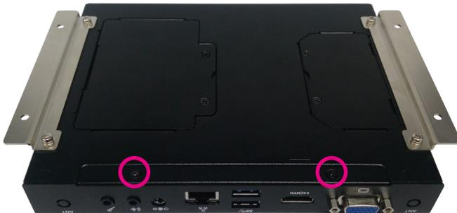
2. Loosen the screws on the VGA connector.
