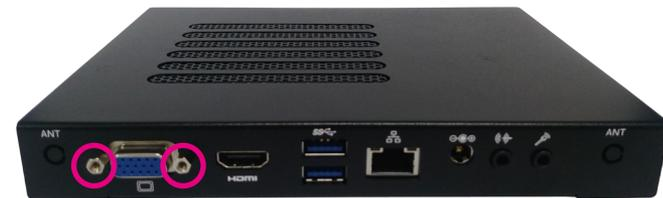
3. With the screws removed, push back the cover and remove it from the chassis.
