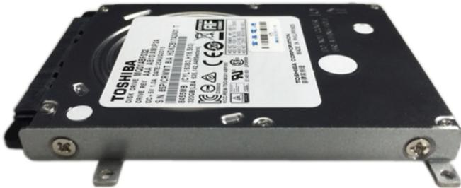
3. Place the SATA drive in the chassis and connect the SATA data connector, then use the provided mounting screws to secure the drive in the chassis.
