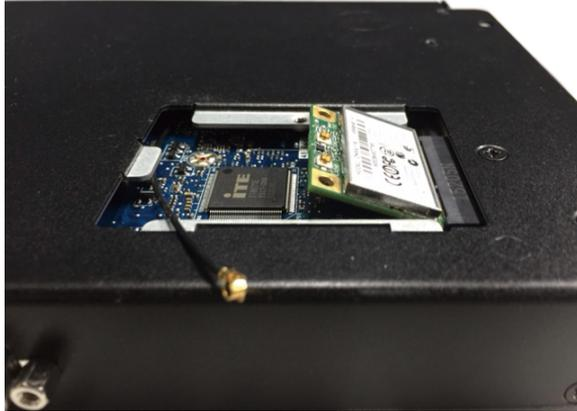
4. Secure the module with mounting screws and attach one end of the RF cables onto the module.
