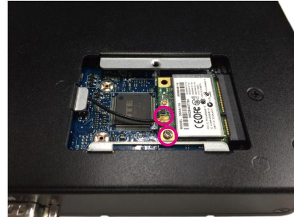
5. Insert the antenna jack end of the cable through the antenna hole.
