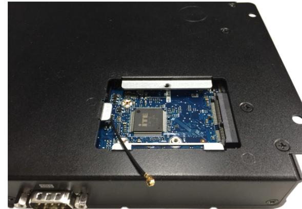
3. Insert the Mini PCIe module into the Mini PCIe slot at a 45 degrees angle until the gold-plated connector on the edge of the module completely disappears inside the slot.
