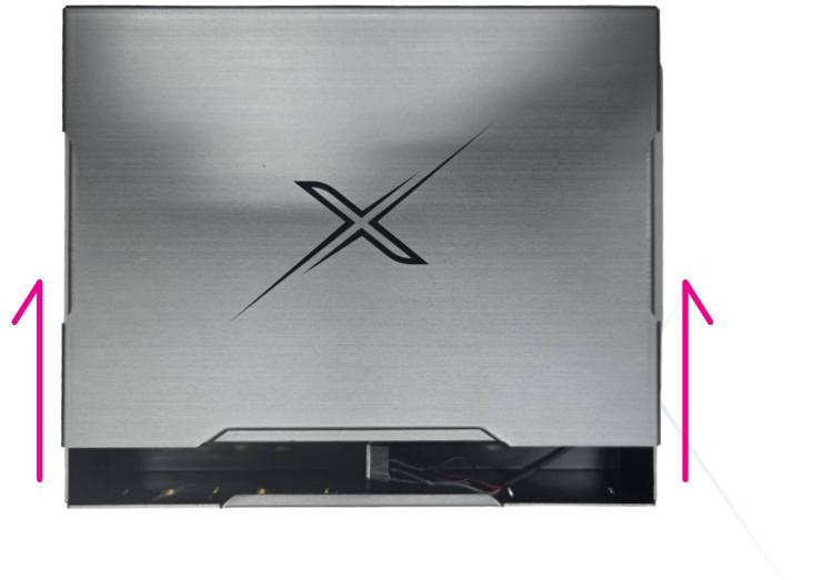
4. Reassemble the top chassis back onto the system once the installation is complete.
