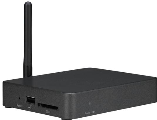
Powered by ARM® Cortex®-A17 quad core, NDiS B115 can play rich multimedia contents with low power consumption. NDiS B115 is enclosed in a compact chassis and can be easily integrated to display devices, such as LCD TV or PDP at site installation with HDMI display output (up to HDMI 2.0 support 4K2K 60Hz), Gigabit LAN. NDiS B115 is suitable as an entry level digital signage player for advertising, messaging, and brand promotion.
