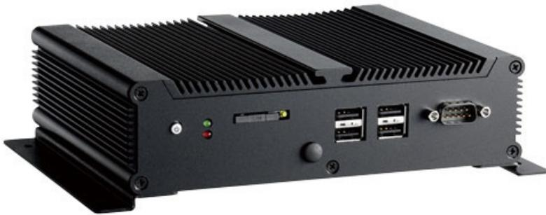
Powered by Intel® Atom™ processor D2700, NDiS 126 has enhanced graphics capabilities to playback HD video with low power consumption. NDiS 126 provides various options of video and audio outputs, dual GbE Ethernet with optional wireless connectivity, SIM Card slot for 3.5G radio connectivity.
