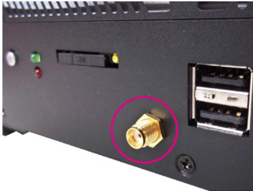
8. Connect an external antenna to the WiFi antenna jack.
