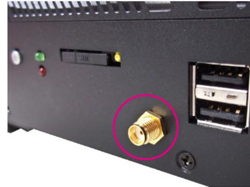
7. Connect an external TV antenna to the antenna jack.
