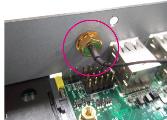
7. The photo below shows the WiFi antenna jack attached at the rear panel of the chassis.
