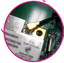
5. Insert the 2 rings (ring 1 then ring 2) into the WiFi antenna jack.
