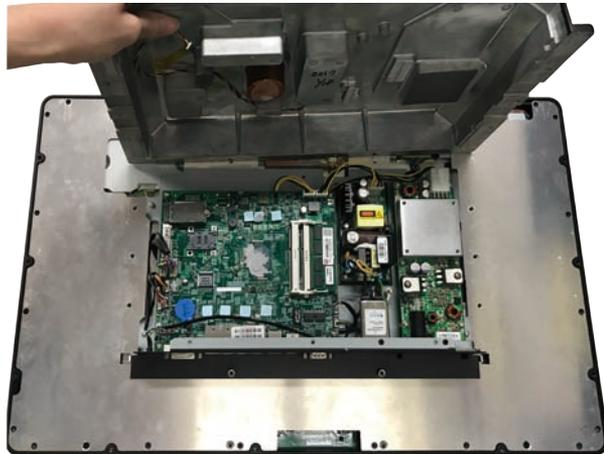
4. Install the Mini PCIe module into the Mini PCIe slot.
