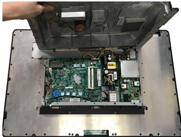
4. Locate the SO-DIMM slot on the mainboard and install a SO-DIMM module into the slot.
