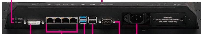
DVI-I    LAN 1 to LAN 4 Ports    USB 2.0    AC Power Socket
