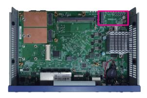
2. Insert the M.2 module into the M.2 slot at a 45 degrees angle until the gold-plated connector on the edge of the module completely disappears inside the slot.
