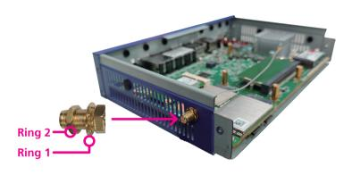
5. Repeat the previous steps to install the other SMA antenna jacks and follow the numbers indicated below to install them into the
