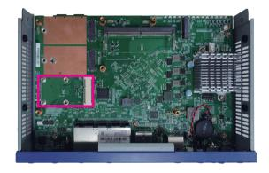
2. Insert the mini PCIe module into the mini-PCIe slot at a 45-degree angle until the gold-plated connector on the edge of the module completely disappears into the slot.
