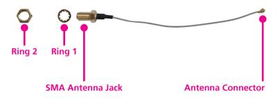
2. Attach the antenna connector to the module's antenna connector.
