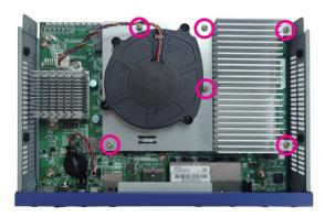
4. Once the chassis and heatsink module have been removed, the system should resemble the image below and be ready for installing extension modules.
