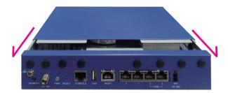
3. Loosen the screws on the heatsink module, place them in a safe location for later use, then lift up the heatsink module.
