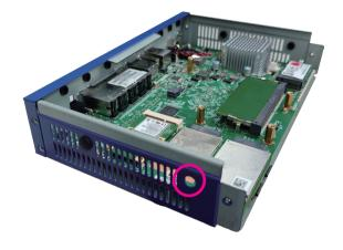
4. Insert the SMA antenna jack through the antenna hole of the chassis, then secure it using the two rings removed in step 1.
