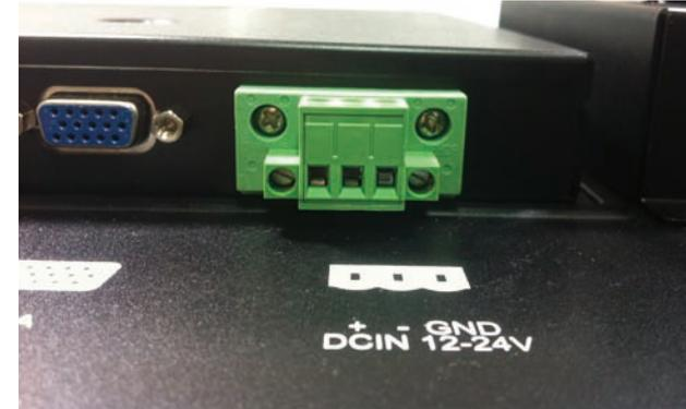
8. Plug the positive, negative and GND wires of the DC power cable into the corresponding pins on the DC input, then tighten the screws on the terminal blocks to secure the wires.
