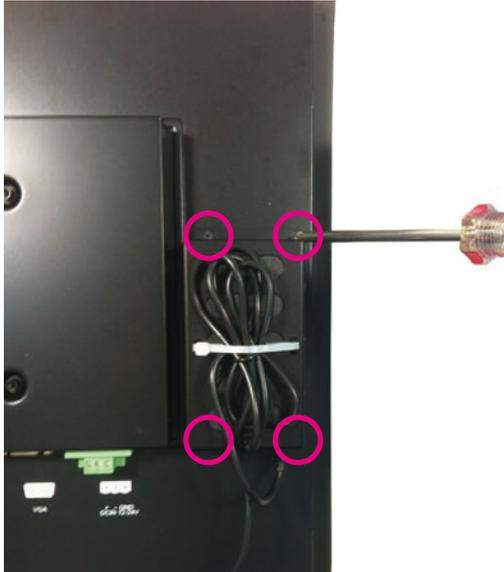
7. Plug the 3-pin terminal block connector into the DC input.
