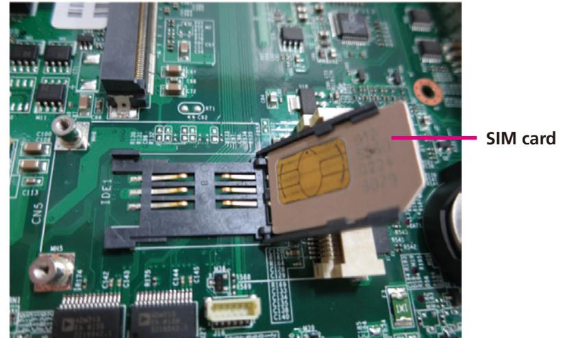
3. Move the holder down and then slide it to the "LOCK" position.
