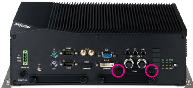
3. Remove the socket's cover to access the CFast socket.
