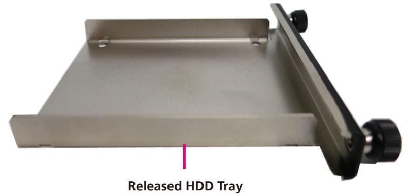
2. Loose both screws to release the HDD tray.
