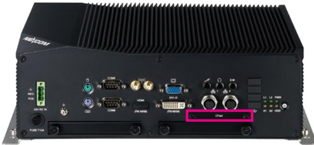
2. Remove the mounting screws of the CFast socket's cover.
