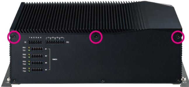
3. Remove 3 screws on the top of the front panel and then put them in a safe place for later use.
