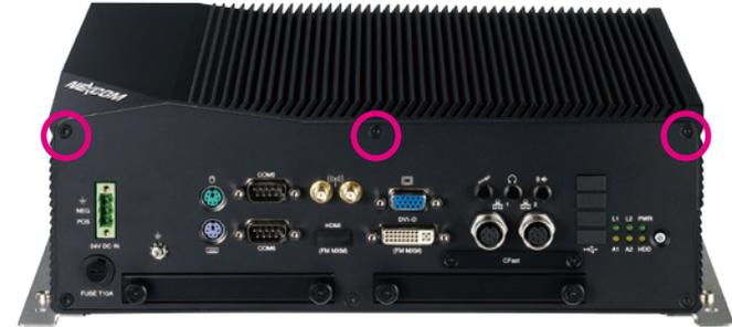
4. Lift up the cover and remove it from the chassis.
