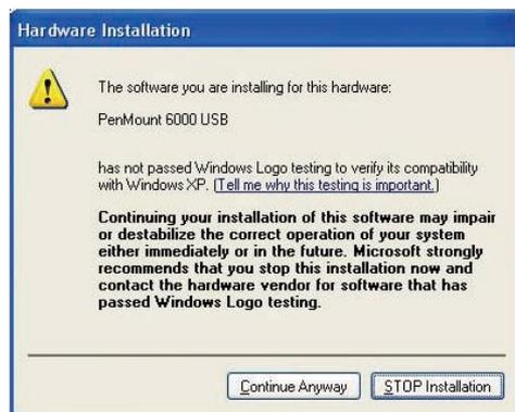
6. When the window below shows up, please select "yes" for installing PenMount as mouse mode; select "no" for digitizer mode. If your operating system doesn't support Windows tablet input, digitizer device can't be used, therefore you have to select "yes" here, otherwise after the installation the touch doesn't work after re-booting.
