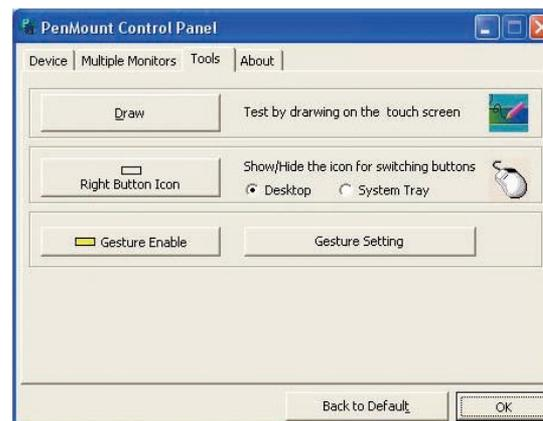
Touch the screen with your finger or a stylus and the drawing screen registers touch activity such **left**, **right**, **up**, **down**, **pen up**, and **pen down**.
