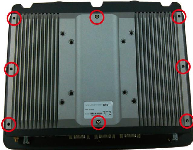
2. Remove the rear cover of the VMC 3000 series. The Mini PCI Express slot shown below is used to install a WLAN module or 3.5G communication module such as GPRS, UMTS or HSDPA module.
