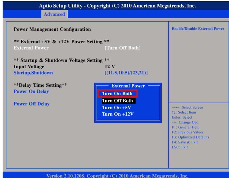
External +12V and +5V Turn Off Simultaneously
