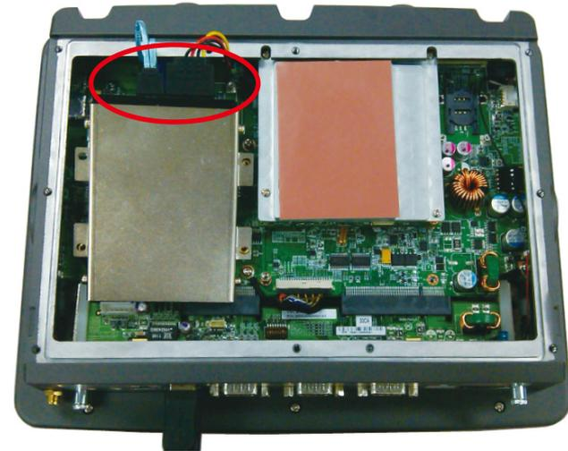
3. Align the mounting holes on the tray to the mounting holes on the board, then tighten the screws to secure the drive to the chassis.
