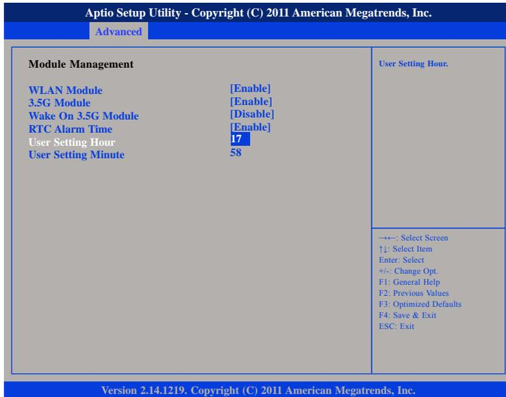
(5) After you have finished with the Setup, press <ESC> to go back to the main menu and then press "Enter" on "Save Changes and Reset."
