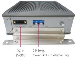
Low Input Voltage Protection Setting
