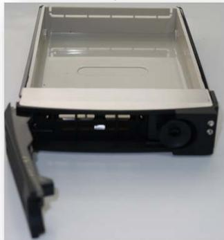
4. Loosen the screws on both sides of the tray and remove the dummy tray.
