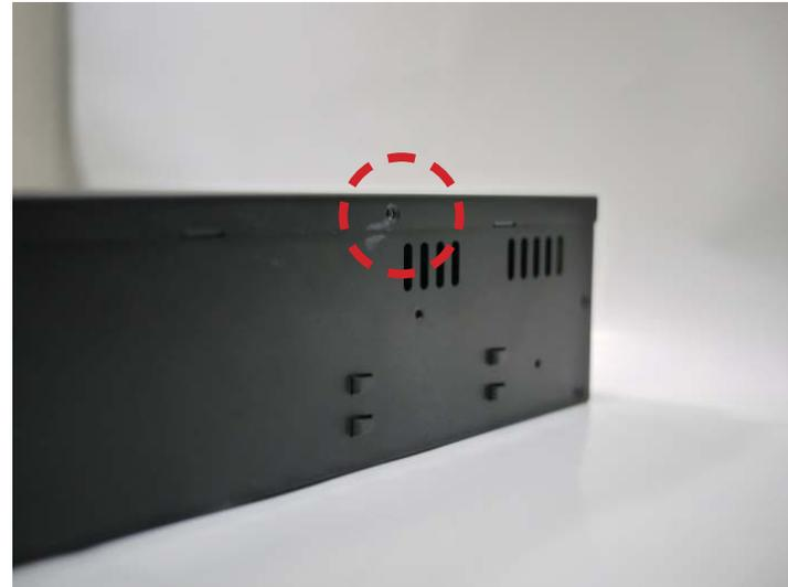
2. Press and hold down the two silver buttons and push the cover forward to slide it off.
