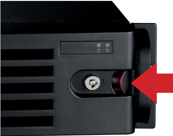
2. Pull the eject button towards right to release the latch.
