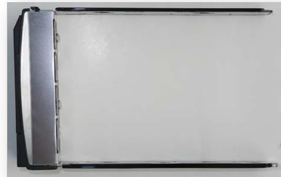
5. Place the SATA hard drive into the tray, and tighten the screws on both sides to secure the hard drive.
