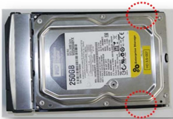
6. Insert the hard drive tray back to the empty slot, and push the latch gently until a click sound is heard to secure the tray.
