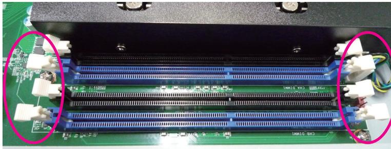
3. Insert the module into the socket at an 90 degree angle. Apply firm even pressure to each end of the module until it slips into the socket.
