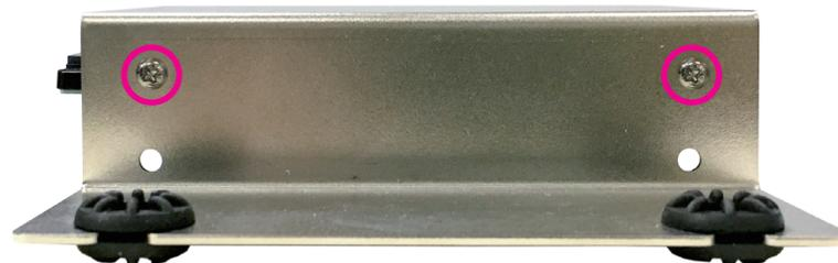
5. Repeat step 4 for securing the screws on the other side of the hard drive bracket.
