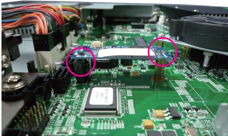
4. Fasten a screw on top of the copper post.
