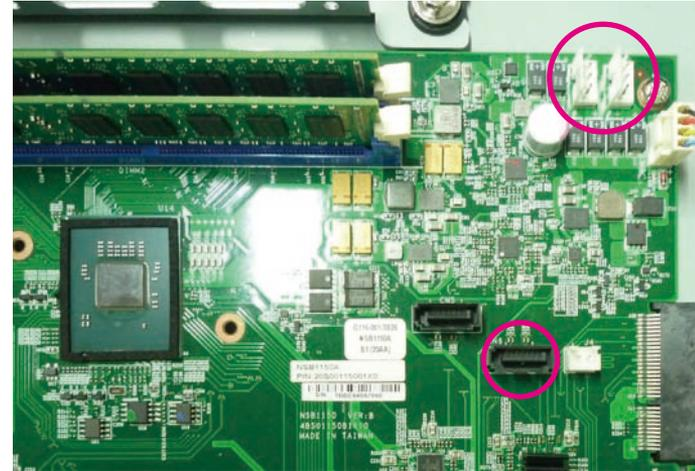
8. Connect the SATA data and power cable onto the board and other ends to the hard drive.
