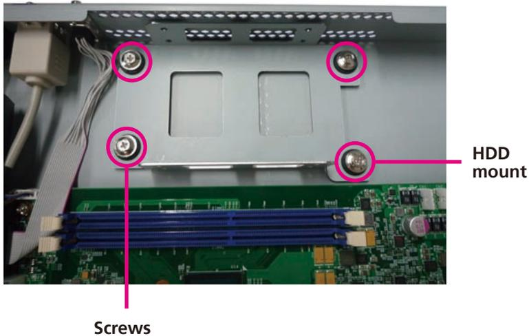
2. Note the sides of the hard drive bracket. When placing the hard drive, make sure the SATA data and power connector are facing the longer side.
