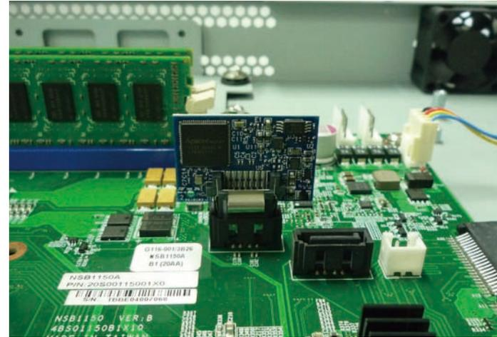
3. Connect the power cable to the SATA DOM power connector on the board.
