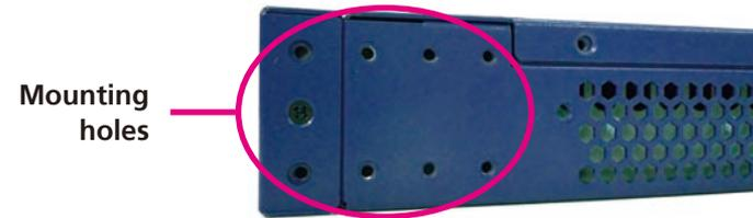
3. Align the mounting holes on the rack ear with the mounting holes on the front panel. Give special attention to the orientation of the rack ear. Secure the rack ear with mounting screws.
