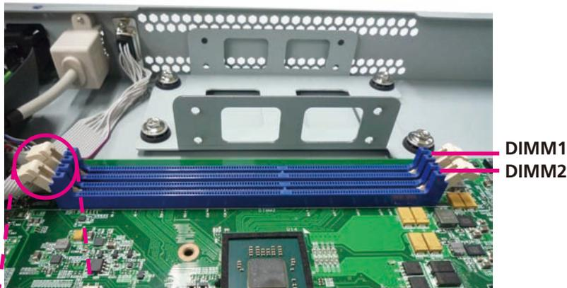
2. Note how the module is keyed to the socket. Grasping the module by its edges, align the module with the socket so that the “notch” on the module is aligned with the “key” on the socket. The key ensures the module can be plugged into the socket in only one direction.
