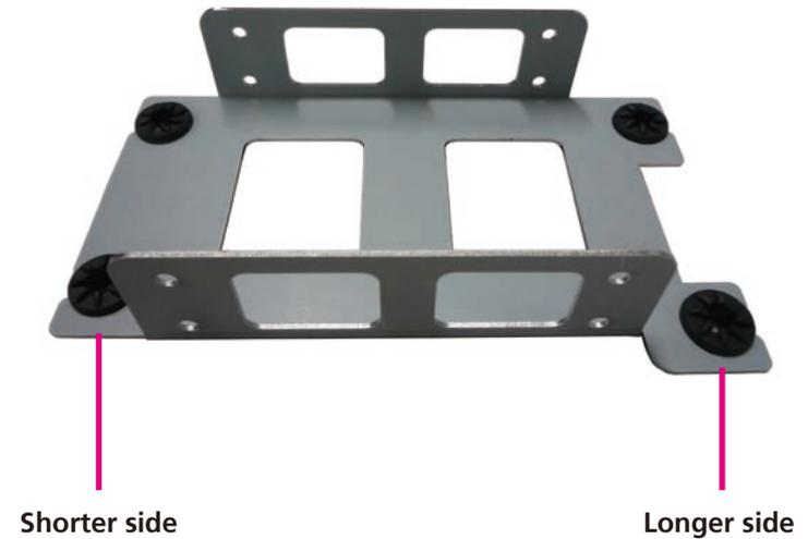
3. Place the SATA hard drive onto the hard drive bracket with the SATA data and power connector facing the longer side.
