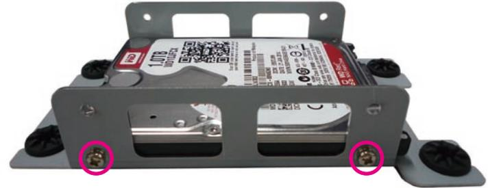
5. Repeat step 4 for securing the screws on the other side of the hard drive bracket.
