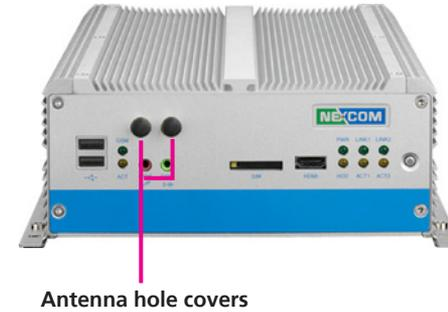
5. Insert the antenna jack end of the cable through the antenna hole. Insert the 2 rings (ring 1 and then ring 2) onto the antenna jack end of the cable.
