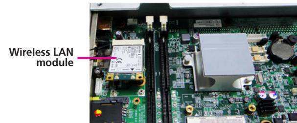
3. Push the module down and then secure it with mounting screws.
