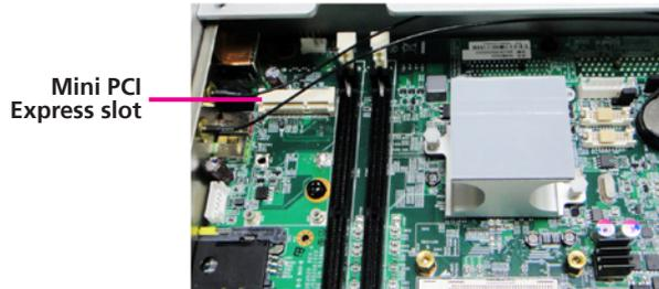
2. Insert the wireless LAN module into the Mini PCI Express slot at a 45 degrees angle until the gold-plated connector on the edge of the module completely disappears inside the slot.
