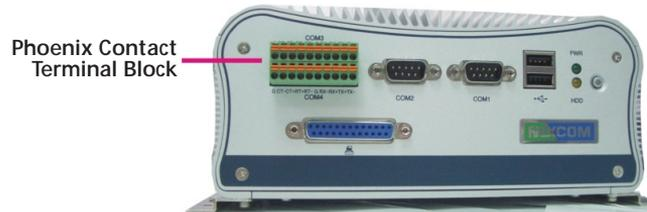
2. Insert a flat-bladed screwdriver in-between the dual bridge rail located in the middle of the terminal block then insert a wire into its corresponding feedthrough.
