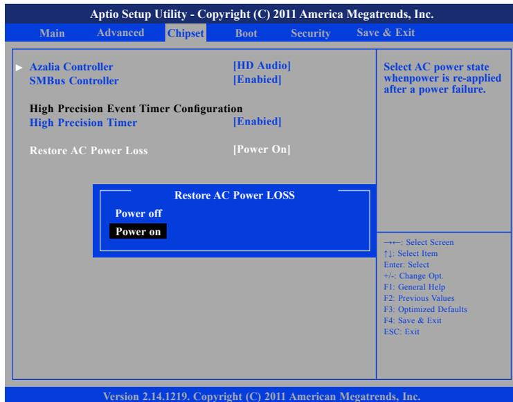
This field is used to configure the AC power state when power is restored after power failure, the options are Power Off and Power On.
