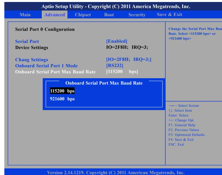
This field configures the maximum baud rate of the serial port 1, the options are 115200 bps and 921600 bps.
