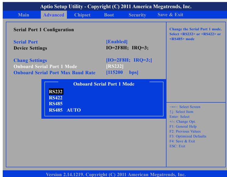
This field is used to configure the mode of serial port 1 as RS232, RS422, RS485 or RS485 AUTO.
