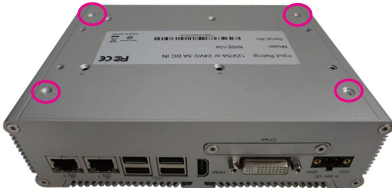
2. Lift up the cover and remove it from the chassis.
