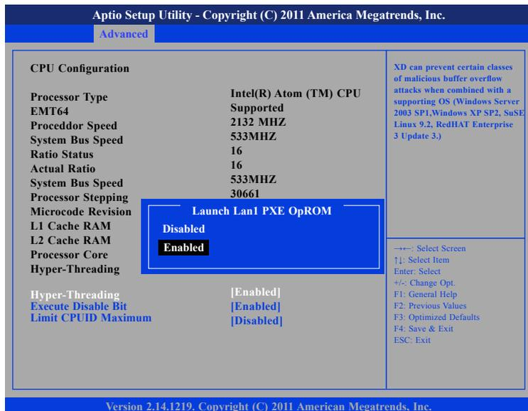
This field is used to enable or disable execute disable bit. When this field is set to Disabled, it will force the XD feature flag to always return to 0. XD can prevent certain classes of malicious buffer overflow attacks when combined with a supporting OS (Windows Server 2003 SP1, Windows XP SP2, SuSE Linux 9.2, RedHat Enterprise 3 Update 3).
