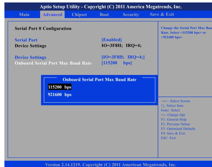
This field configures the maximum baud rate of the serial port 0, the options are 115200 bps and 921600 bps.
