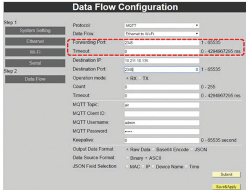
This setting is used to setup the Ethernet TCP configuration. In this mode, Ethernet is a TCP server, while Wi-Fi is a TCP client.
