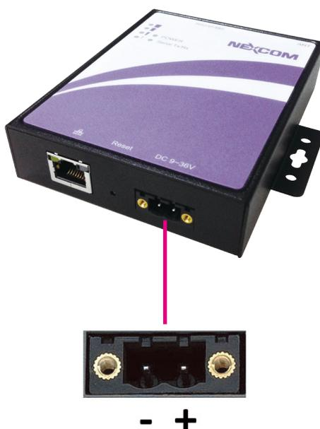
1. Prepare DC power source (9~36 VDC) or NEXCOM optional power adaptor accessory.
