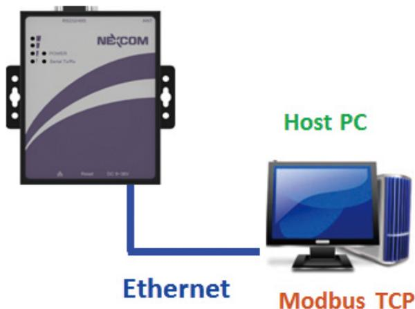
1. Make sure the network settings on the Host PC are correctly configured so that NIO 50 and PC are on the same subnet.
