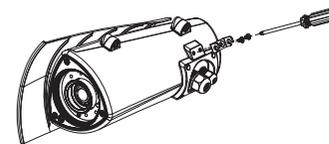
5. Press and hold down the latch on the wall mount bracket and put it into the connecting bracket. Once in place, secure the other side using the supplied hex wrench.
