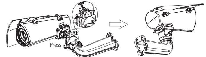
6. Align the mounting holes on the wall mount bracket to the mounting holes on the wall mount plate, then secure it tightly with screws to finish the installation.
