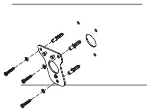
4. Secure the connecting bracket to the camera's rear.
