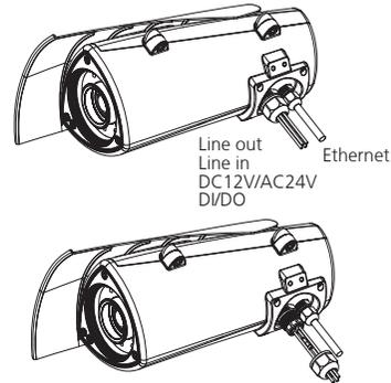
3. Open the camera's cover and glue the dehumidifier packet onto the metal bracket using the adhesive sticker on its back, as depicted in the diagram below. Close the camera's cover and ensure the clip is locked in position. Install the sunshield and tighten a torx screw on the side of cover.
