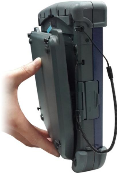
3. Connect the auxiliary battery to the system using the captive screws in the auxiliary battery.
