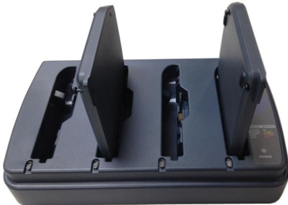
3. Plug the AC power cord into the nearest electrical outlet and then plug the other end to the battery charger's DC jack located at the rear of the battery charger.
