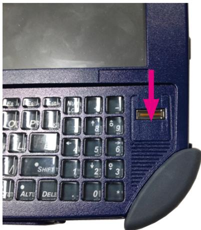
The biometric mouse performs two functions, security and screen navigation (simulating a mouse). Use the F9 function key to toggle between the two features.
