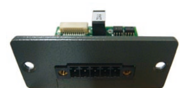
Universal PROFINET, EtherNet/IP and EtherCAT I/O Bracket
