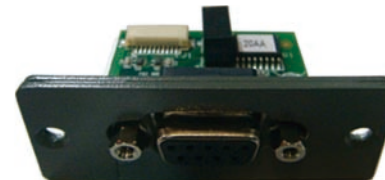
Universal PROFINET, EtherNet/IP and EtherCAT I/O Bracket
